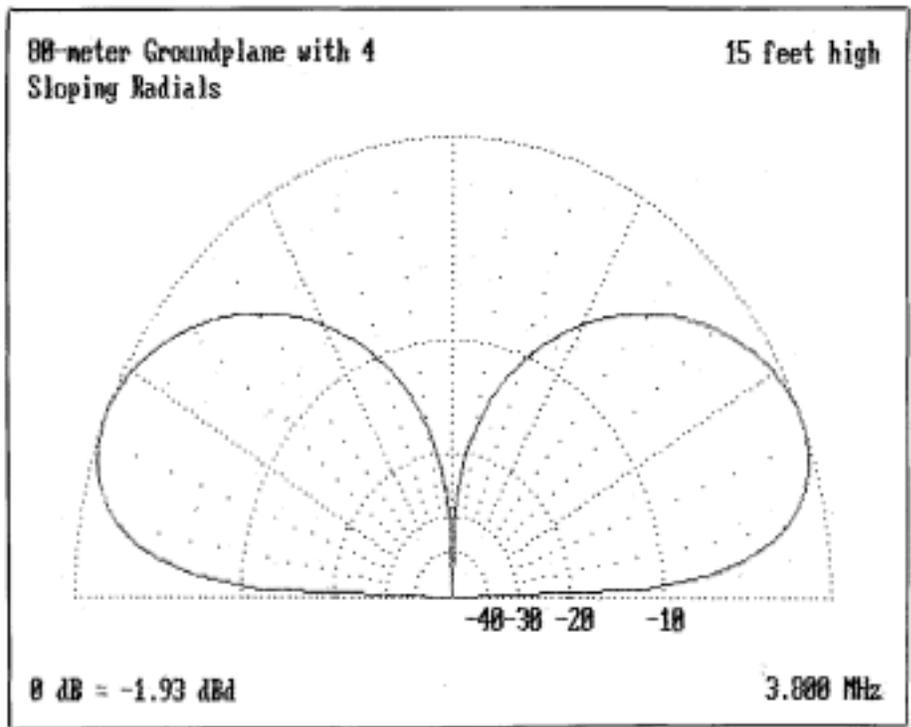
Fig. 6- Groundplane with four radials, .06 wavelength above ground at base. Polar plot of radiation angle.
