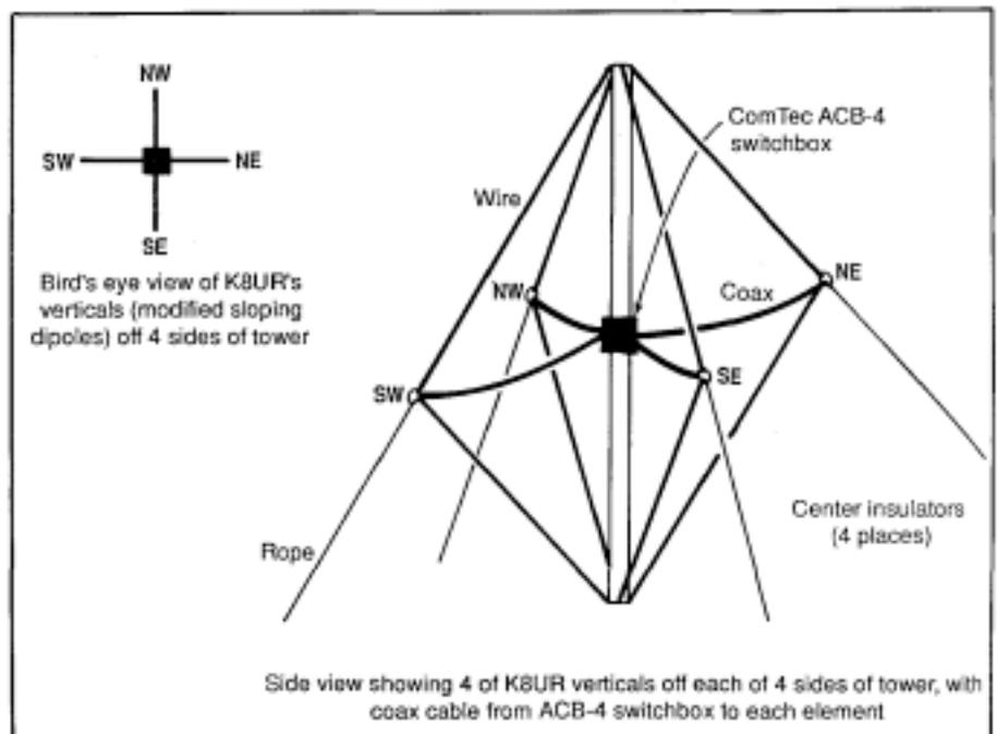
Fig. 7- Four-square setup using K8UR verticals.
