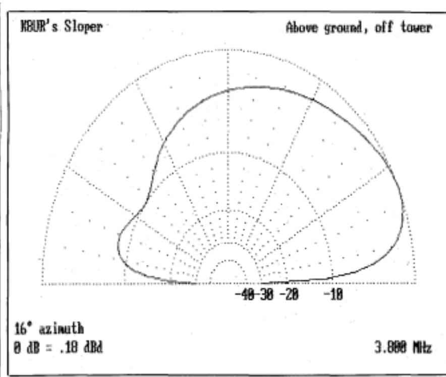
Fig. 1- Sloping dipole polar plot of radiation angle with 120 foot tower support.
