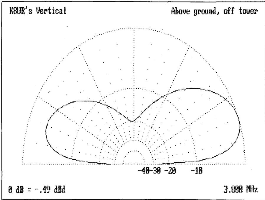
Fig. 4- K8UR vertical polar plot of radiation angle with 120 foot tower.
