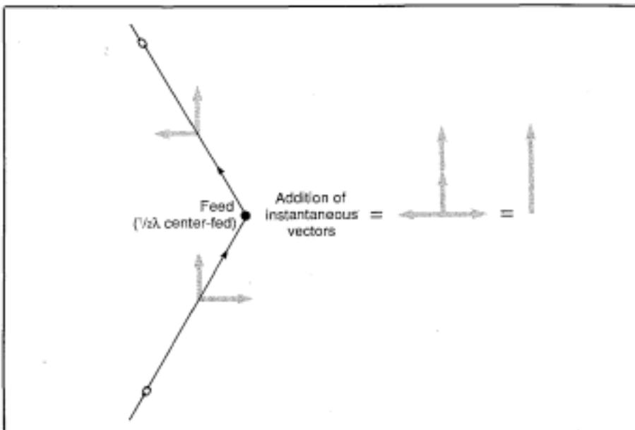
Fig. 5- Current vectors for K8UR vertical showing vertical addition and horizontal cancellation.
